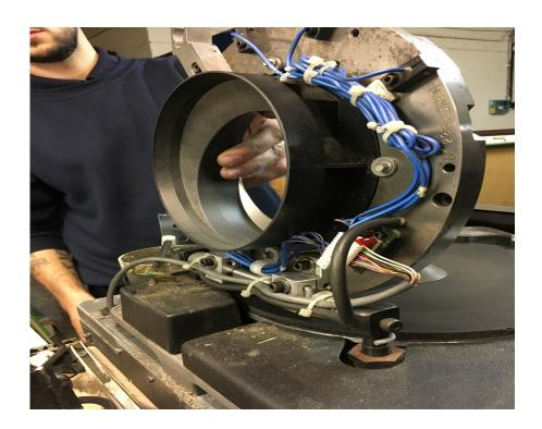
Once you have got the head secured and lying flat, remove plastic cone from center of the rubber mat with an Allen key
