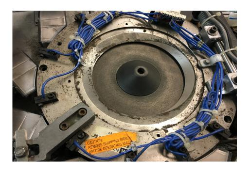
Place wooden template sent back with head into center of turntable while it is locked down and insert Allen key bolt into center and tighten. This will center the head
