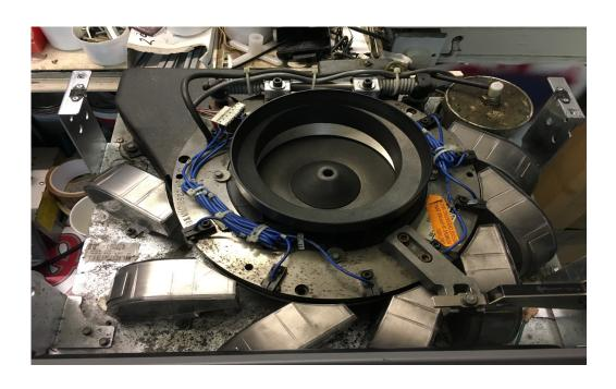
Remove 4 bolts on spring loaded hinge with Allen key the easiest way to do this is with the head in an upright position as shown
